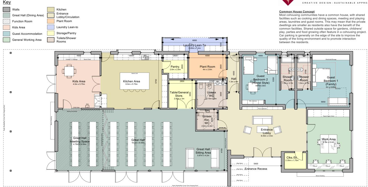
Proposed Common House Floor Plan - Approx Internal Area = 385m<sup>2</sup> (Gross Area = 416m<sup>2</sup>) Scale 1:100
